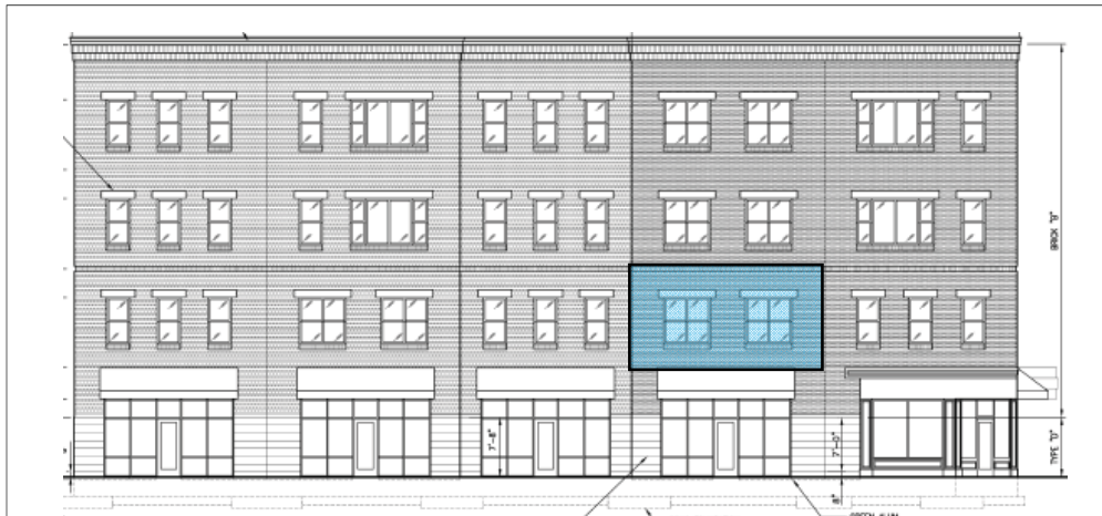
Figure 33– Panel #5, Erection Sequence-4; Located Along 3 rd Street
